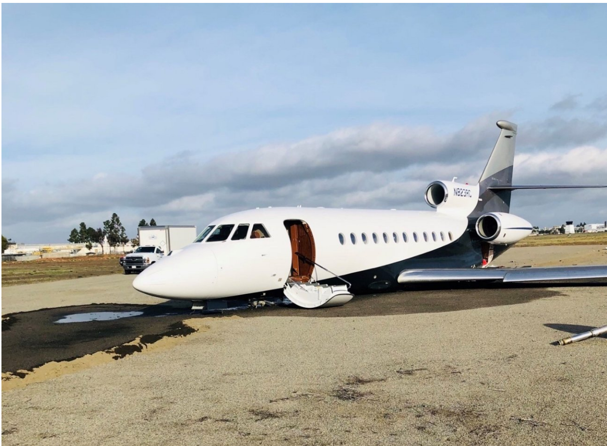
Figure - View of Airplane Damage (Source: FAA)
